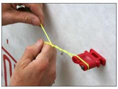
5. Place the twisted loop over the second ALINE-SET. Pull and feed the line around the ALINE-SET until tight.
