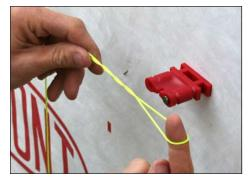
4. Twist the loop two to three times.
