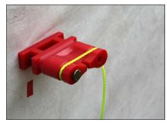
2. Tie your line to the first ALINE-SET using a simple loop with slip knot.
