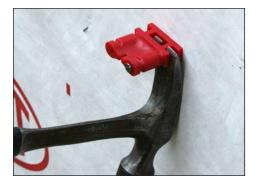
When finished, pull the line from the notch and remove, then easily remove ALINE-SETs with your hammer claw.
